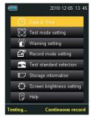
4.2.2 When the selected item has been set up, press the "RETURN / LIGHT" key once to exit the menu. Press the "RETURN / LIGHT" key again, then the detector will return back to the real-time data collection display page, and the detector entered set up state.
