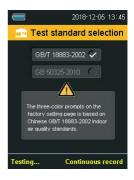
4.7.2 After the setting has been finished, press the "RETURN/LIGHT" key once to exit the "test standard selection" item and the detector will automatically store the data that has been set.
