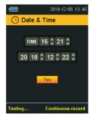
4.3.2 After the setting has been finished, press the "RETURN/LIGHT" key once to exit the date and time setting. Press the "RETURN/LIGHT" key once again, the detector will return back to the real-time display page of data collection and automatically store the data that has been set
