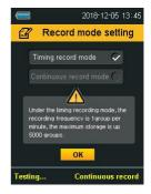
(Kindly reminder: under the fixed-time record mode, the information recording frequency of the detector is 1 group per minute, and the maximum information recording are 5.000 groups!)
