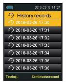
4.12.3 After record check has been finished, press the "RETURN/LIGHT" key to exit the "History records" item. Press the "RETURN/LIGHT" key once again, the detector will return back to the real-time data collection display page and enter setting accomplished state, then return back to the data display interface.
